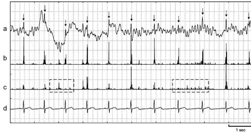
Figure 1.22: ECG artifacts distort the raw EEG signal (adopted from Joe-Air Jiang, et al., 2007).
