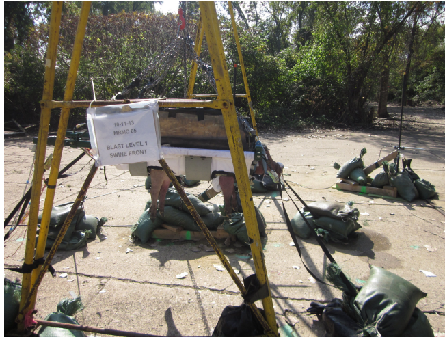
Figure 2.1: Instrumented swine test: the pig head was front to the blast wave
