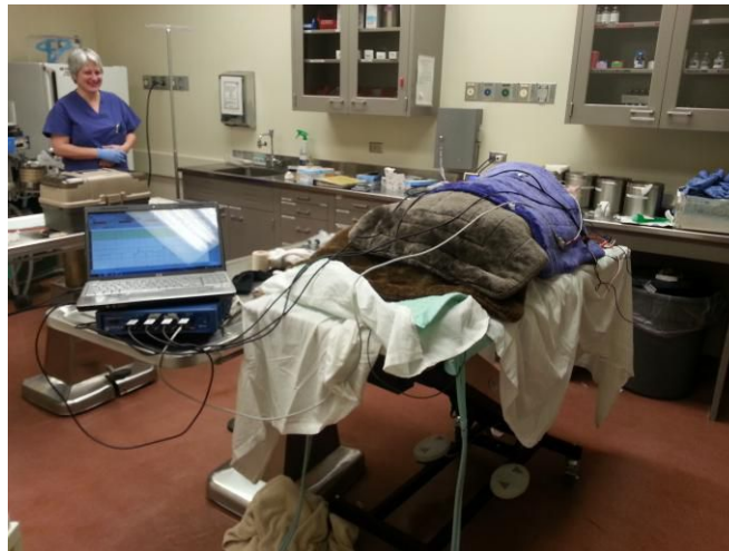
Figure 2.2: 4-channels Biopac data acquisition system (MP-36) connects to the computer via a USB port.
